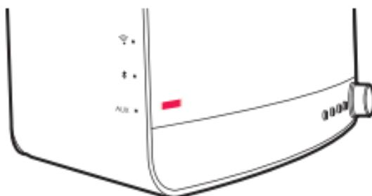
The battery is running low on charge. After flashing, the indicator goes out after a while. If you press the INPUT button on the front of the main unit in this state, the indicators flash to indicate that the battery charge is low.
